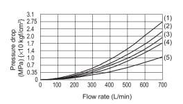
Pressure - Flow rate characteristics
