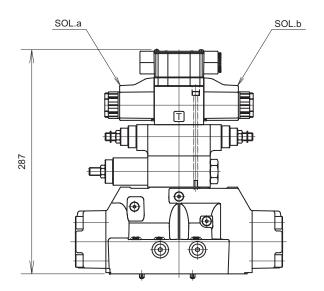
With MT-02W-60 (type W) (Hexagon socket head cap bolts used: M5 x 85, 4 pcs.)
